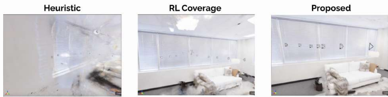
Figure 6: Novel view synthesis from the same held-out camera pose. Heuristic (18.79 dB PSNR) fails to reconstruct scene geometry. RL Coverage (33.05 dB) recovers structure but retains blur. Proposed (33.33 dB) produces the sharpest reconstruction with 25% fewer views.
