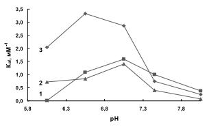
**Fig. 6.** The pH dependence of immobilized lipase activity on the surface  $(1) - \text{KAU}_{OX}$ ,  $(2) - \text{SKN}_{OX}$  compared with native lipase (3)
