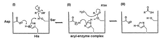
Fig. 4. Scheme of catalytic R-C(O)-XR' substrate hydrolysis by lipase [11]
