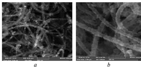
Fig. 2. SEM images of CNT-1CeO<sub>2</sub> (*a*) and CNT-20CeO<sub>2</sub> (*b*) samples
