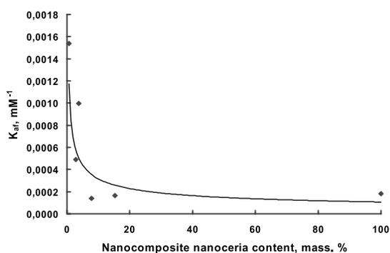
Fig. 8. Dependence of nanocomposite catalase-mimetic activity on nanoceria content under pH 10.5
