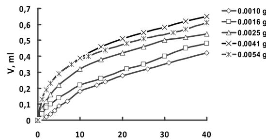
Fig. 4. Kinetics of H<sub>2</sub>O<sub>2</sub> decomposition with different catalyst amounts
