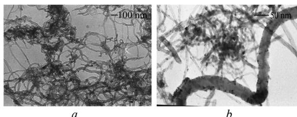
Fig. 1. TEM images of pristine (*a*) and modified (*b*) CNT
