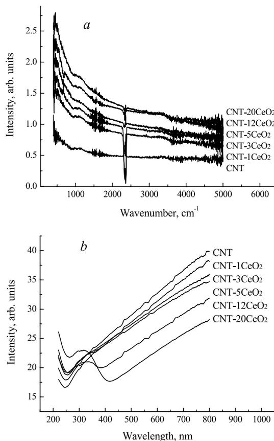
Fig. 3. Nanocomposites IR (*a*) and UV (*b*) spectra
