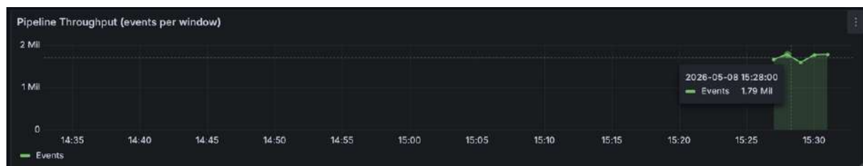
Figure 4.1: Grafana pipeline health panel at 10,000\times replay speed: throughput plateaus at approximately 1.79 million records per minute, indicating that the data producer — not the Kafka or Flink layers — is the binding bottleneck at this configuration.
