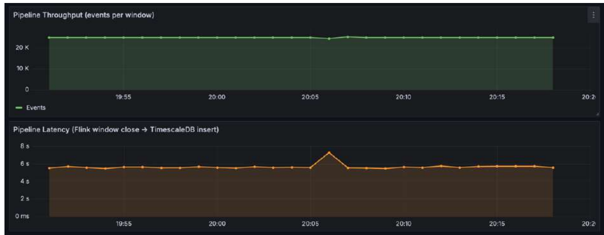
Figure 3.8: Pipeline health panels: throughput (events per 60-second window) and end-to-end latency (window close to TimescaleDB insert).
